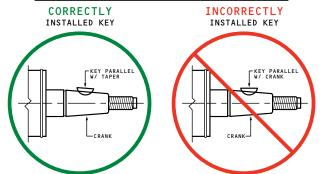
INSURE FLYWHEEL BOTTOMS ON TAPER, FLYWHEEL SHOULD NOT WOBBLE WHEN PROPERLY SEATED. BE SURE TO PROPERLY TORQUE FLYWHEEL TO MANUFACTUREB'S SPECIFICATIONS.
